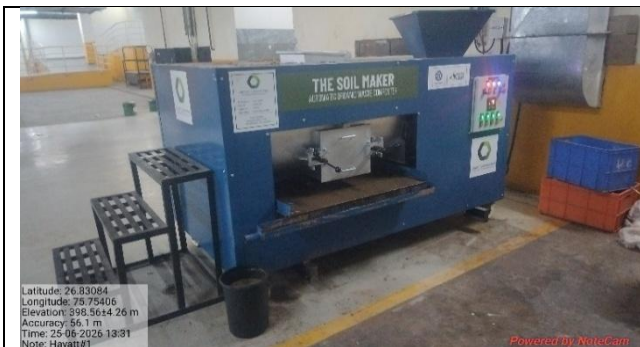
Organic waste Compost machine and compost generation at Hyatt Residency
